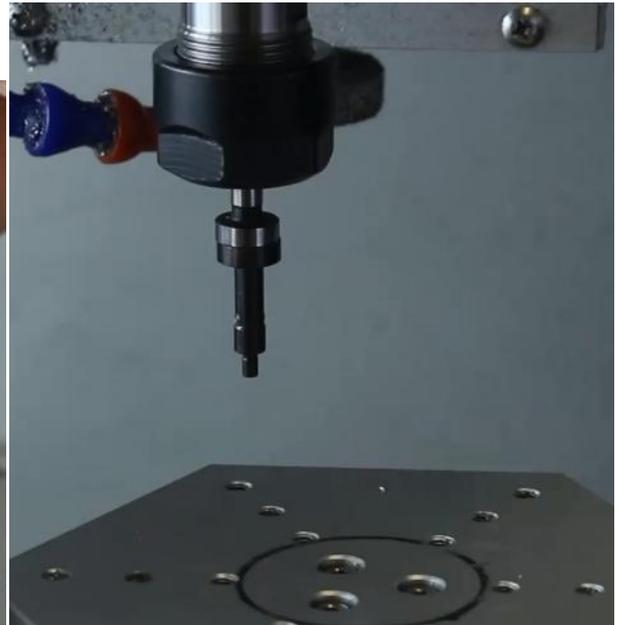
Secondly , Y Axis starting point setting , Moving the edge finder to the front of the Axis table ,and then Zero Y Axis , Moving it to other side , The MACH3 software show the total edge finder traveling area. The Y Axis starting point was the middle point . Normally, The number was 78. At last , Moving the spindle to 78.000, and Zero Y Axis . The Y Axis starting point was finished .
