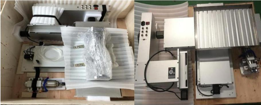
1.2 Place the upper part on the base, Tighten the screws at the bottom of the base
