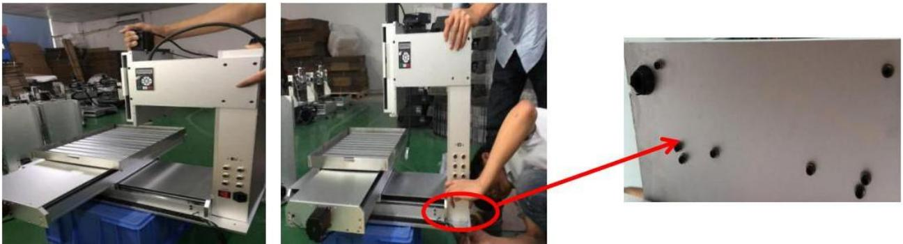
1.4 Open the cover of the vertical part, then tighten the screws around the stepper motors. Close the cover.
