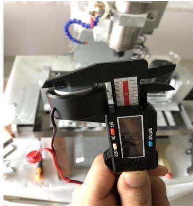
3, Then enter the height of the sensor into the offset
