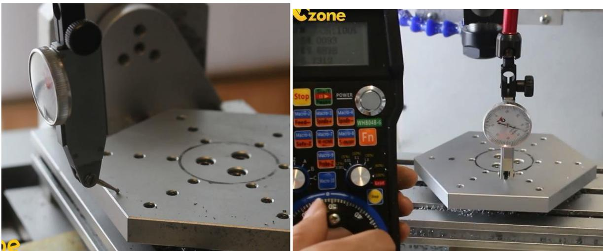
Remark: if not level, You can rotate B Axis angle to adjust and keep it level.
