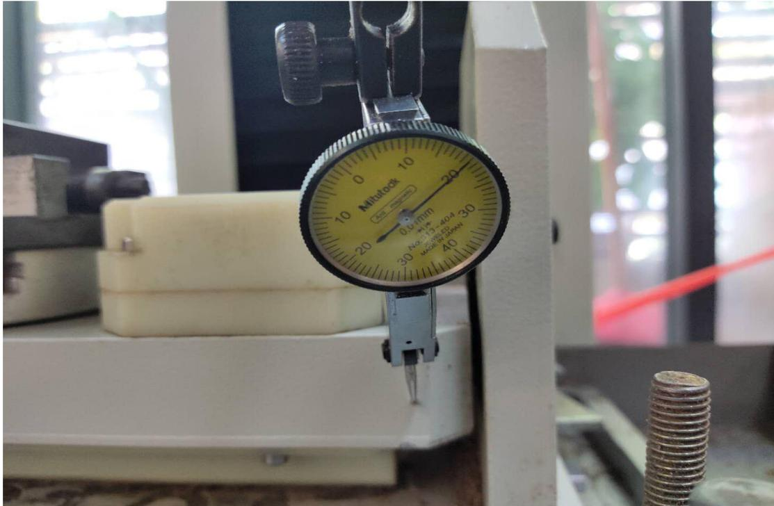
**Note:** If it is not parallel, I hope you can use a soft thing to rap the 5-axis table to adjust the position, for example, with a wooden hammer, do not use hard things to hit the table or it will damage the 5-axis table.
