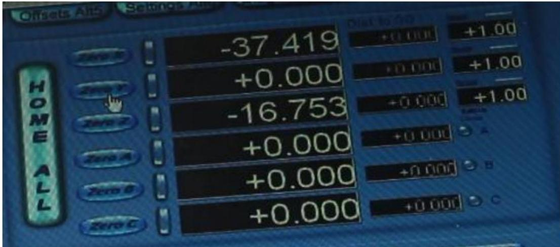
Divide the total stroke value by two, shake the Y-axis to "the value obtained by dividing by two" and click the Y-axis to clear.
