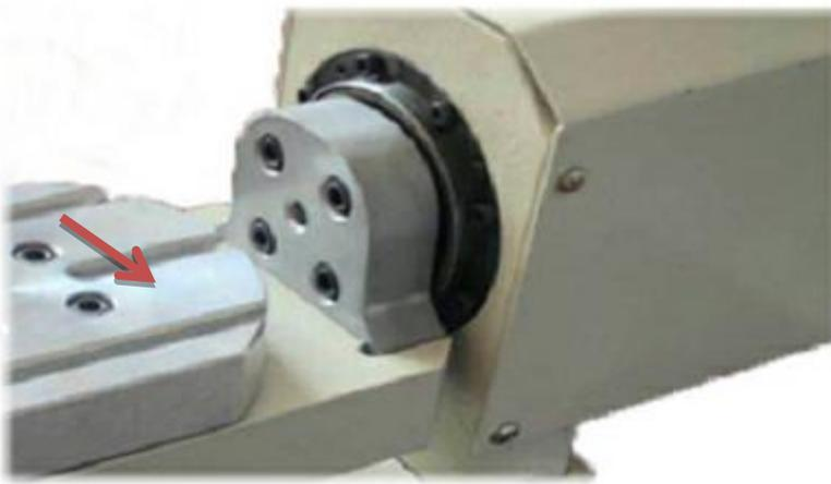
5. The tool touches the direction indicated by the arrow, then click Z to clear, the Z-axis starting point is completed.
