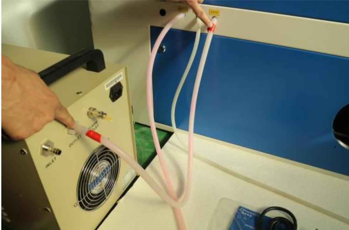
B. Connect WATEROUT tube with INLET port in CW3000 chiller, as below picture.
