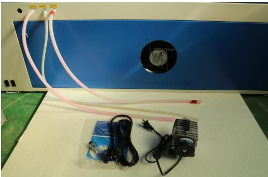
A. Connect WATERIN tube with OUTLET port in CW3000 chiller, as below picture.
