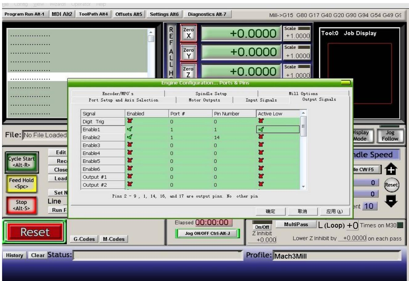
9. Spindle setup in “Ports and Pins” menu to click “Spindle Setup”, set as below, and then save.
