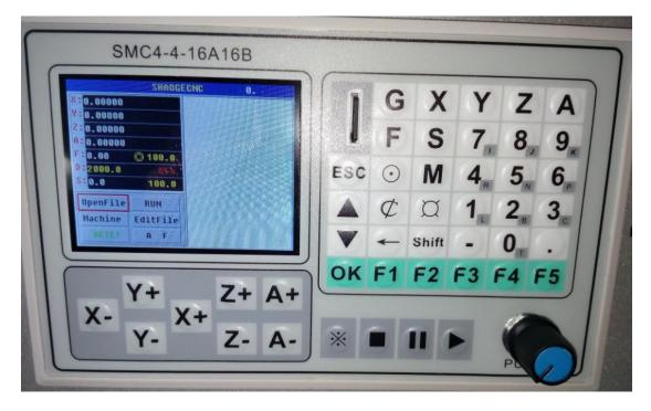
The DSP system has high quality requirement for TF card , Did not use cheap and low fake TF card . Suggest use such as Kingston , Sandisk , Samsung and so on famous brand TF card. Then The DSP system only can recognize 50 pcs different G code.
