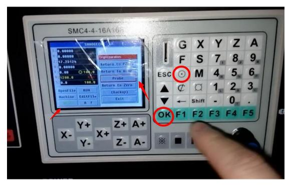
Then ,The engraving bits will touch probe ,and bounce back , take probe
