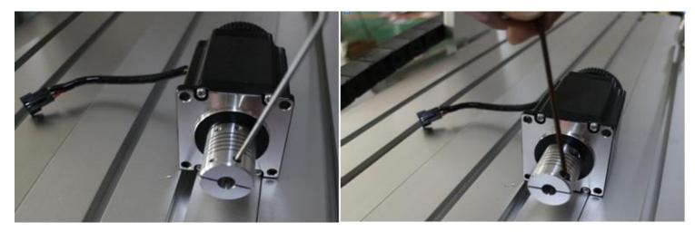
Third, tight the screw of coupling, make sure ball screw and couple good contact.
