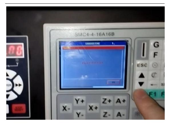
Select G code setting ,and filled with offset numbers in probe blank.
