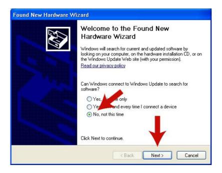
Driver installation will complete when the CNC USB Controller is connected to the USB Port. Windows XP will detect controller hardware and the 'Found New Hardware Wizard' will launch. Use of 'Windows Update' is not required.
