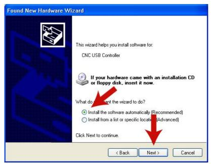
The new hardware wizard will present additional options. 'Install the software automatically' is the recommended option. Press 'Next' to continue, or 'Cancel' to stop installation.
