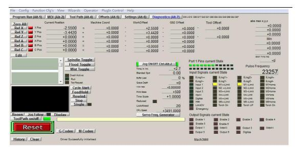
Then using probe to touch engraving bits ,The below one will get black ,and the other one will get light, ,The test is finished ,it shows the probe hardware connection is correct.
