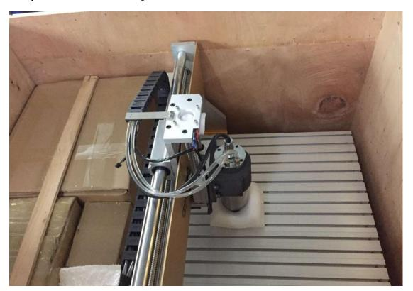
2. Then unpack wooden box , the machine is almost assembled. Only need to install step motors and water pump. All step motors are same for  $X\ Y\ Z\ Axis$ . At first, Put step motor to corresponding Axis. Tight the four screws and make sure tighten. Connected that corresponding cable.
