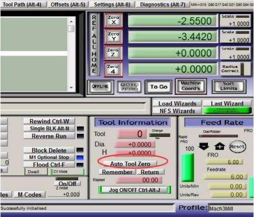
At last, Take probe away from work piece, Click Goto Zero button, The machine will automatic go to zero point. The start point setting is finished.
