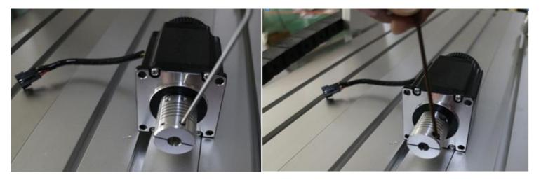
tight the screw of coupling, make sure ball screw and couple good contact.
