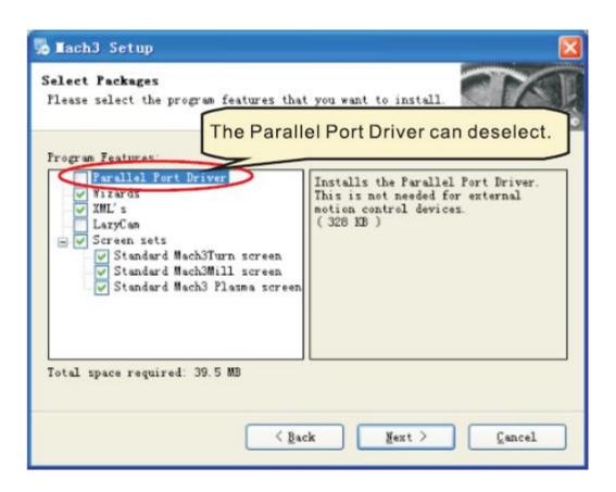
After installation finished ,Connect USB cable between controller box and computer. Copy NcUsbPod.dll from USB card driver file to MAC3/PlugIns file .This file to enable USB motion
