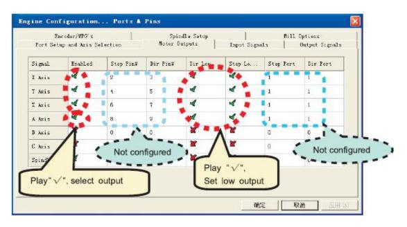
Motor parameter settings, X Y Z Axis setting is completely same ,The Axis setting is different.
