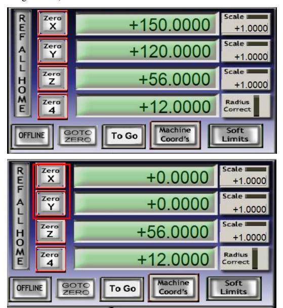
Put probe under spindle again, click auto zero tool again , The Z Axis will automatic touch probe and return back , Meanwhile Z Axis will Automatic Zero Z .
