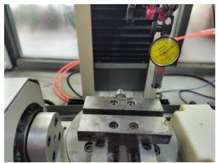
If it is not parallel, you can rotate the angle of the A-axis table to adjust and keep it parallel.
