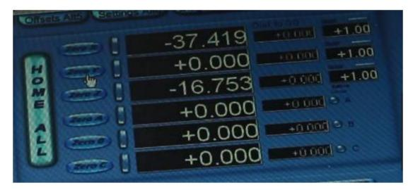
Divide the total stroke value by two, shake the Y-axis to "the value obtained by dividing by two" and click the Y-axis to clear.
