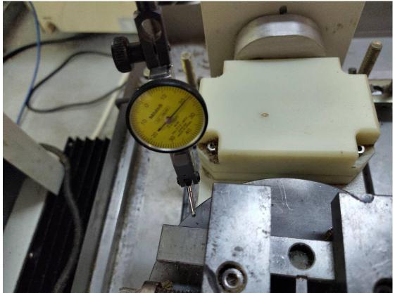
4. If it is not parallel, you can rotate the angle of the B-axis table to adjust and keep it parallel
