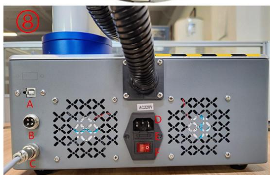
A: USB Port C: Foot port E: Spare fuse B: Rotary axis port D: Power Cable F: Main switch
