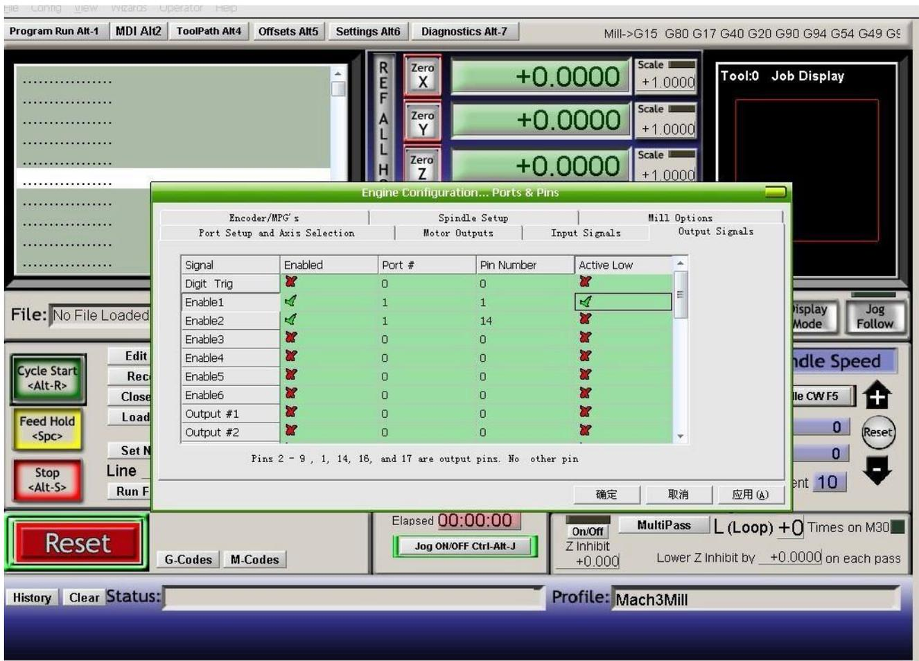
9. Spindle setup in "Ports and Pins" menu to click "Spindle Setup", set as below, and then save.
