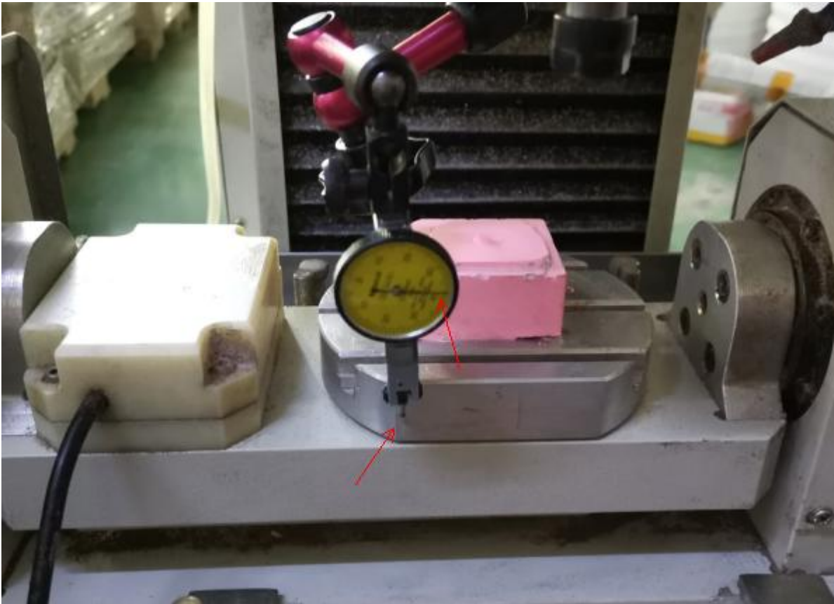
Use the handwheel to adjust A axis as follow:
